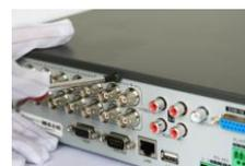
2. Install the HDD on the chassis
