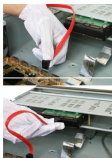
4. Connect the power cable to the HDD.
