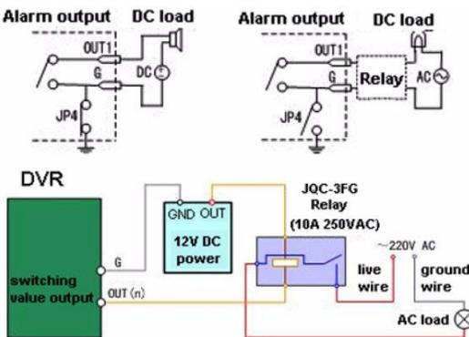
For DC load, JP4 can be used within the limit of 12V/1A safely. If the interface is connected to an AC load, JP4 should be left open. Use an external relay for safety (as shown in the
