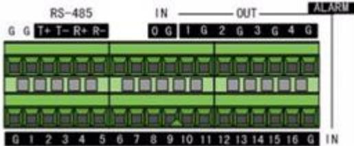
The alarm input is an open/close relay. If the input is not an open/closed relay, follow the connection diagram below:
