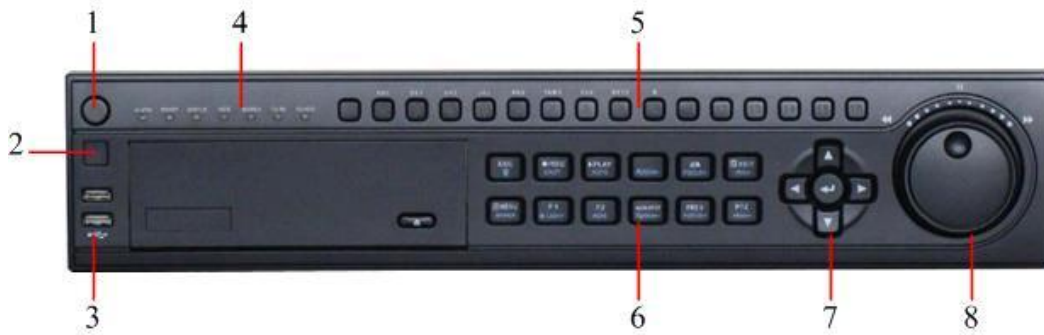
Figure 3. DVR Front Panel Controls
